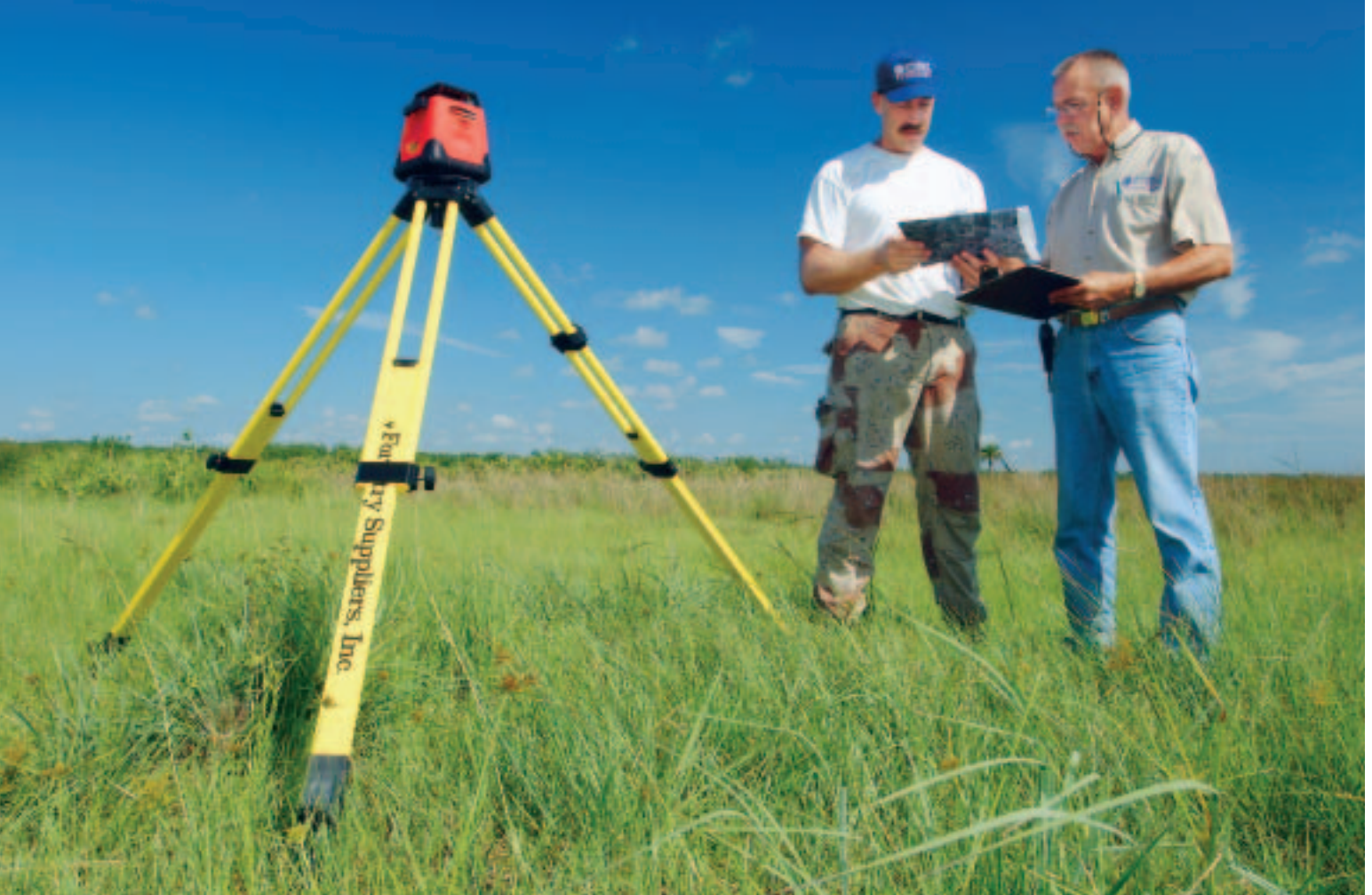
Mark Clark, left, a research assistant professor in UF's soil and water science department, and Mitch Flinchum discuss a wetland elevation survey and placement of a water control structure near Lake Okeechobee. The red instrument on the yellow tripod is a laser leveling system that is used with a Global Positioning System to determine the elevation contour and water storage capacity of an isolated wetland near the lake. (Photo by Eric Zamora)
